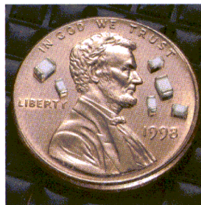
High Frequency Ceramic Inductors
